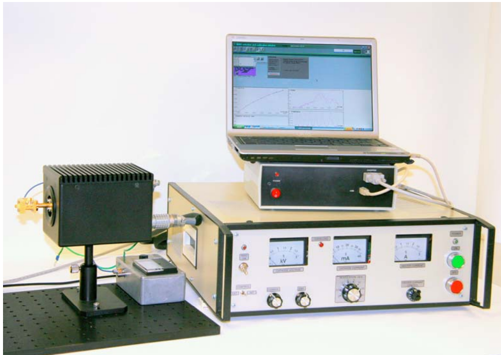
Figure 1: QS2-1000 THz source, VR-3M power supply and DAU-1 unit
